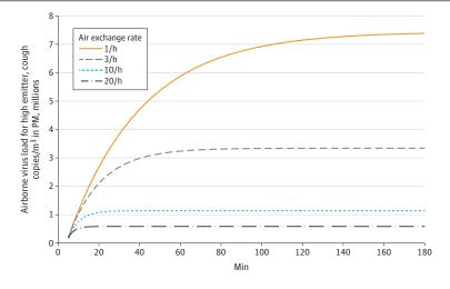
The simulation estimated the concentration in a closed room for different air exchange rates. The emitter was assumed to have a high virus load in the lungs and to be coughing intermittently every 30 seconds.
