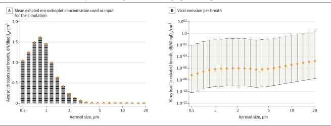
A, The typical exhaled microdroplet concentration used as input for the simulation. B, The modeled viral emission per breath for typical (orange), high, and low (whiskers) emitters.  $dN/dlogD_n/cm^3$  is the number concentration normalized by the aerosol size-bin width.
