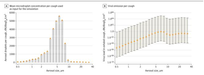
A, The typical exhaled microdroplet concentration used as input for the simulation. B, The modeled viral emission per breath for typical (orange), high, and low (whiskers) emitters. dN/dlogD<sub>n</sub>/cm<sup>3</sup> is the number concentration normalized by the aerosol size-bin width.
