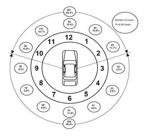
Figure 16 - PTW usually in Driver line of sight prior to collision Diagram from MAIDS<sup>15</sup> & reproduced with the permission of ACEM
