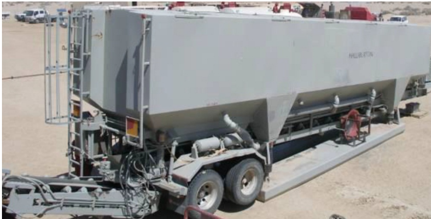
Figure 11: Sand Trailer Unit (Halliburton, 2012)
