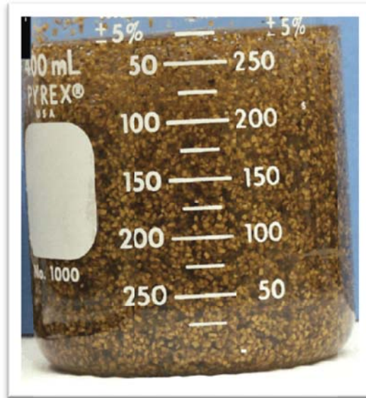
Figure 20: Typical Sand - Guar Gum fluid mix (Source Economides and Martin, 2007)
