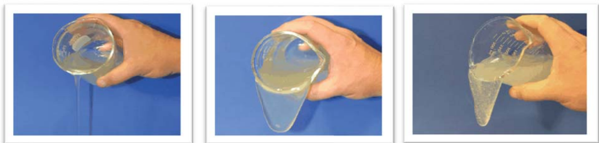
Figure 18: Example of Typical Stages of Gum (Guar) Cross-linking to Achieve 300 cp (Source Economides and Martin, 2007)
