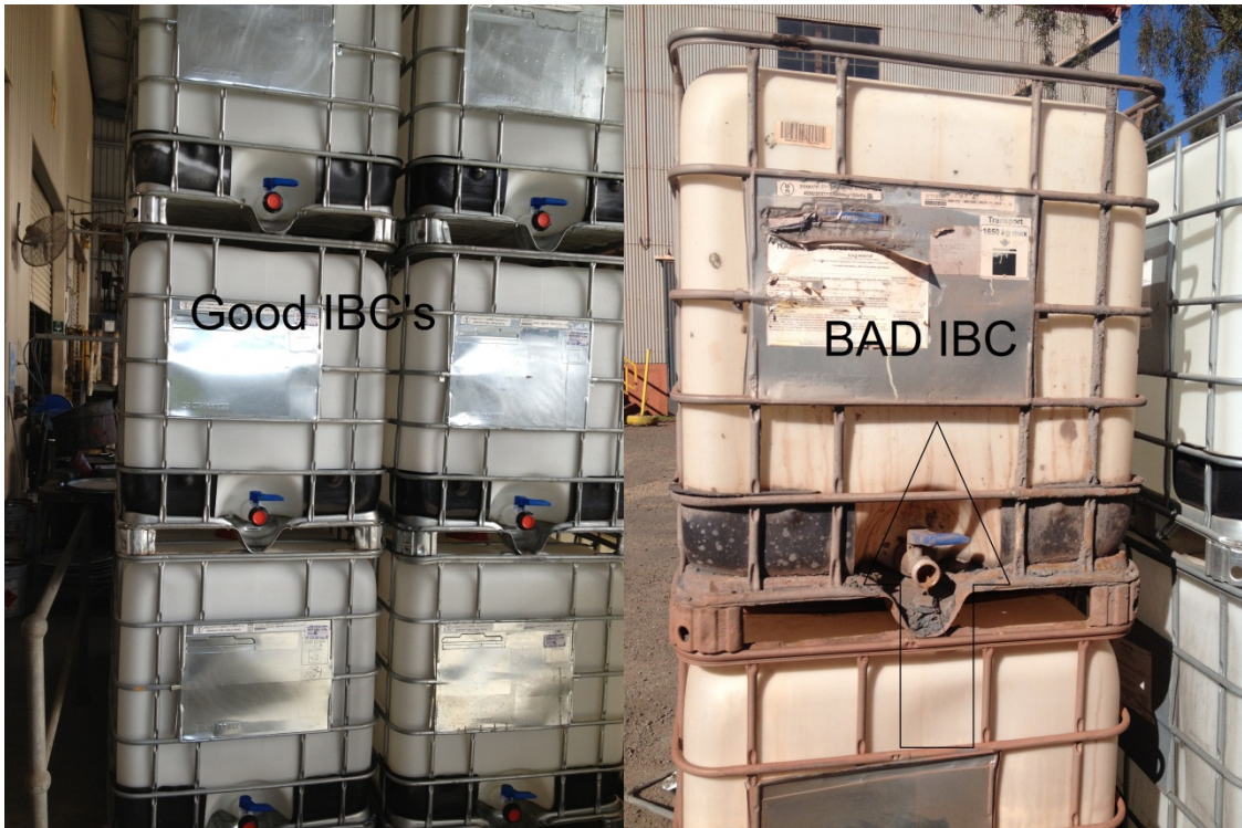
Photo 1. Example of IBC in good condition. Photo 2. Example of IBC in poor condition
