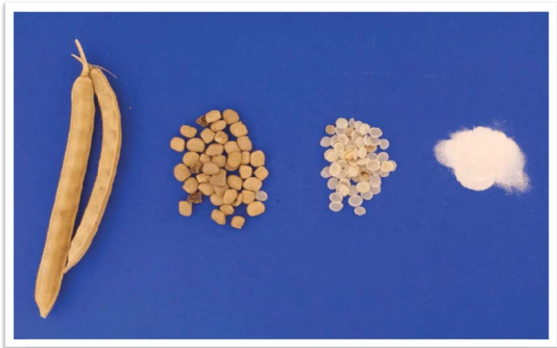
Figure 17: Example of a typical slurry gum constituent, Guar Gum – illustrating its native form, seed form, splits and powder
